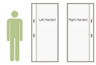
BBGs are typically handed so that the operators are located opposite the patio door handle on operating sash and opposite the center mull on the fixed sash.
